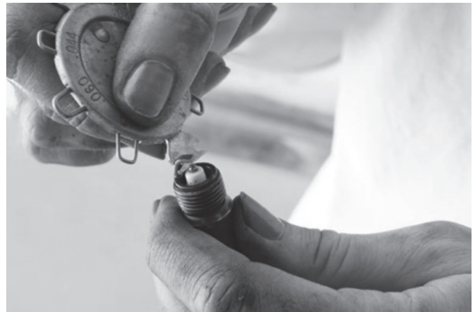
Figure 5-19. Adjust Spark Plug Gap
